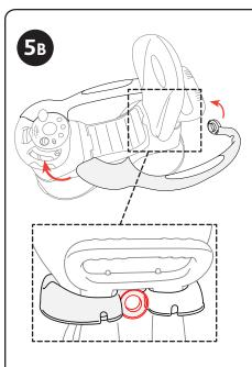
5B. Attach the Left Side Armrest (G), fit the ring on top of the Right Side Armrest ring at the back of the Backrest and onto the Steering Wheel.
