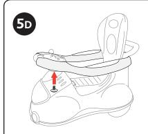
5D. Secure the Left and Right Armrest with a small Armrest Screws (H) under the Steering Wheel as shown. Use a coin to tighten the screws.
