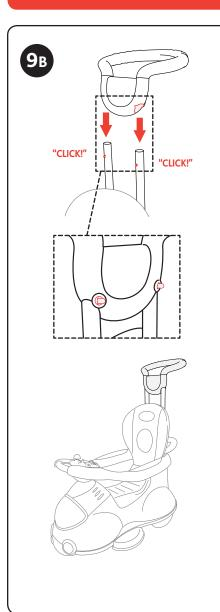
9B. Attach the Parent Handle (K) to the Extension bars. Line up the bars and push down until they click into place.
