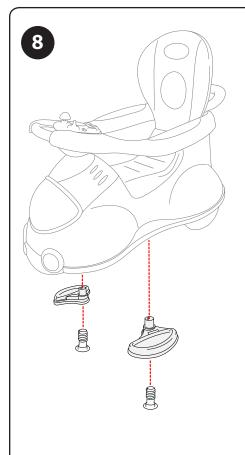
8. To create the Push 'n Go Mode: Remove Left and Right Rocking Base and replace them with the Left and Right Footrest (J). Secure the Footrest with the same screws, tighten with a coin.
