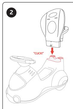
2. Line up the Backrest/handle for Child (C) to the Car Body as shown and push down until you hear it click into place. Pull up on the Backrest to make sure that it is securely attached to the frame.
