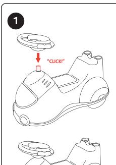
1. Attach Steering Wheel (B) to Car Body (A) as shown. The Steering Wheel can only be attached in one direction. Push down on the center of the Steering Wheel until you hear it click into place. Pull up on the Steering Wheel to make sure it is securely fastened to the frame.
