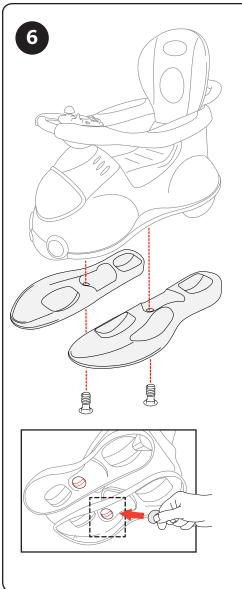
6. Attach Left and Right Rocker Base (E) as shown. Secure them with Rocker/Footrest Screws (F) as shown. Use a coin to tighten the screws.
