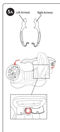
5A. Attach the Right Armrest (G) first, fit the ring into the back of the Backrest and onto the Steering Wheel.
