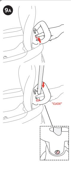
9A. Insert both Extension Bars (L) into the back of the Backrest as shown. Slide the tab over to open, insert the Extension Bar and push down until it clicks into place. Repeat for the other side.
