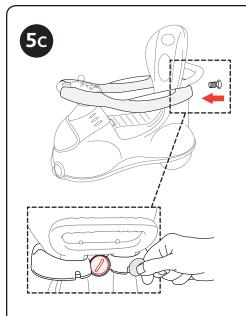
5C. Insert the largest Armrest Screw (H) into the back of the Backrest, through the Armrest rings. Use a coin to tighten the screws.
