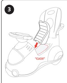
3. With the Seat (D) in a vertical position, attach it to the frame as shown. It will click into place on both sides of the seat to create a hinge, for access to the storage compartment under the Seat.
