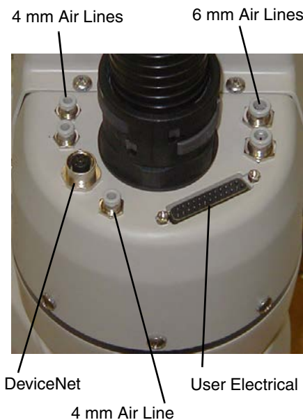
Figure 6-3. User Connectors on Joint 2
