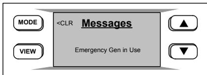
Press the **VIEW** button again to display the “Messages” screen. This screen allows the user to view any text messages sent from the control system (Only when part of a Cresnet system).
