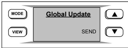
Pressing the **MODE** button again displays the Global Update screen. Allows a single thermostat location to update the current temperature settings to all other thermostats on the system.
