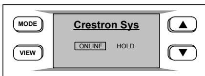
Pressing the **MODE** button again displays the Crestron System screen.
