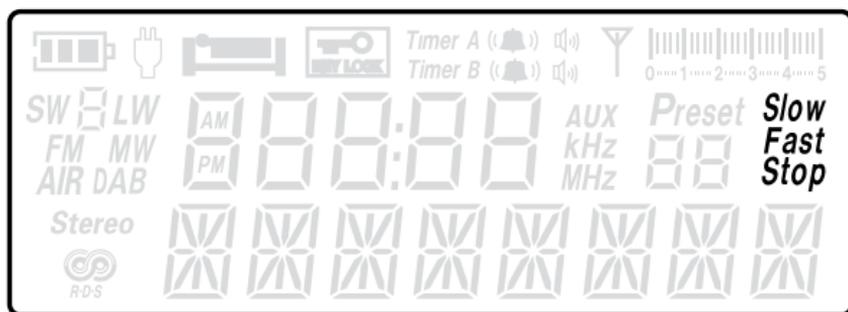
For "SLOW" mode, rotate tuning knob to increase or decrease frequency for FM at 10kHz, MW at 1kHz, SW at 1kHz;
