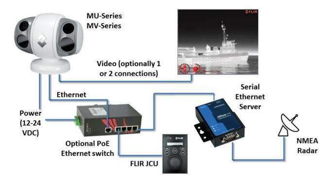
Important: Per the warning above, the Ethernet connection from the camera is connected to the unpowered (non-PoE) port of the PoE switch. The switch shown has one unpowered port and 4 powered ports. Alternatively, it would be possible to use a non-PoE Ethernet switch, and use PoE Injectors to power the JCU and the Serial to Ethernet Server.
