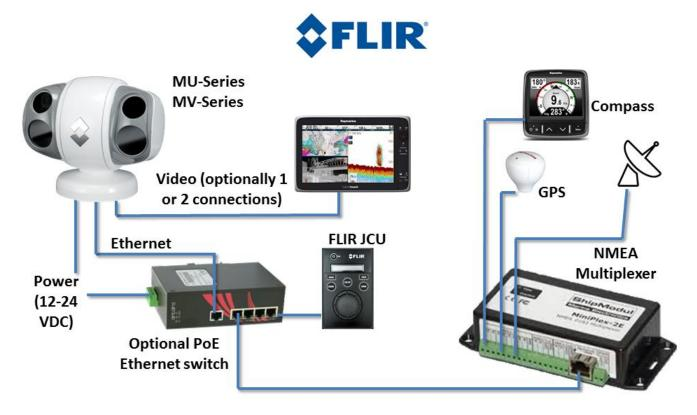
Connect the ShipModul mux to power and to the switch. Use the MPX-Config tool that comes with the device to search the network and locate the device. Then change the IP address to one that is compatible with the camera and other equipment. In this example, the ShipModul mux uses 192.168.250.94.
