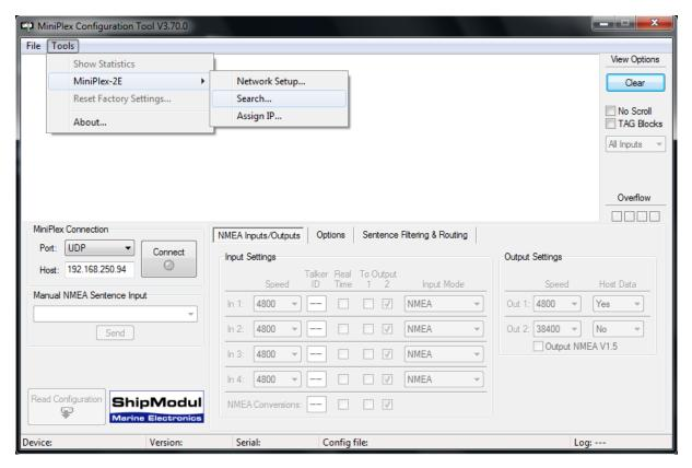
The ShipModul uses port number 10110, which is a registered port for NMEA data. Therefore the UDP Terminal of the Radar Server configuration is also set up to use port 10110. Open the camera server.ini configuration file with a text editor, as in the first example. Perform a search of the file for "Sensor 1" to locate the section related to the UDP Terminal:
