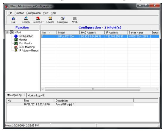
Use the Configuration option to set the Serial parameters to match the radar. For example, NMEA 1083 specification uses a baud rate of 4800.
