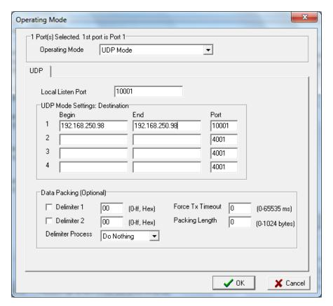
Set the UDP Mode Settings Destination Begin and End IP addresses to the IP address of the camera, and set the port number to 10001. These correspond to the UDP Terminal that is configured in the Radar Server.
