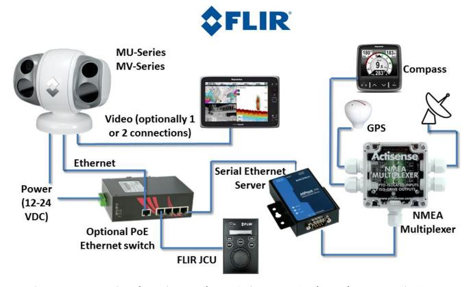
As in the previous example, refer to the manufacturer's documentation for configuration and wiring information about the serial ports on the NMEA mux, Serial Ethenet server and other devices. Specifically, ensure that both sides use the same signalling standard (RS422 or RS232), baud rate, and so on. Ensure the transmitted signals from the NMEA devices go to the receive side on the NMEA mux. Similarly, ensure the transmit signals from the NMEA mux go to the receive side of the NPort server.
