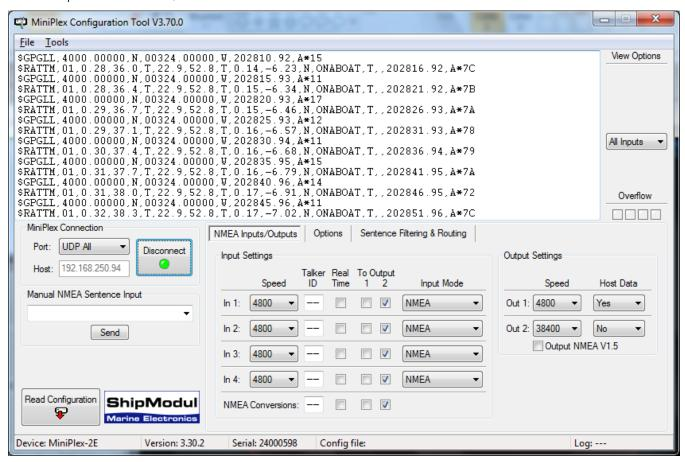
Verify if the mux is receiving NMEA data from the devices. The image above shows \$GPGLL sentences from the GPS and \$RATTM sentences from the radar.
