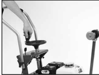
(B) Lower the CX-3® to its lowest position.
