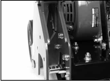
(D) Locate the three Blade Guard Retaining Bolts.
