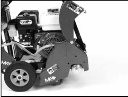
(A) Remove the Diamond Blade. See Blade removal section.
