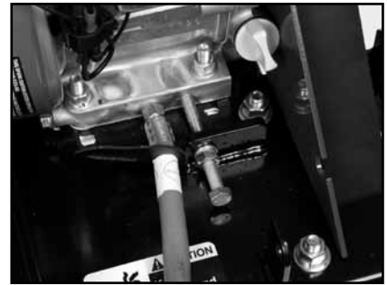
(L) Tighten the Motor Tension Arm.
