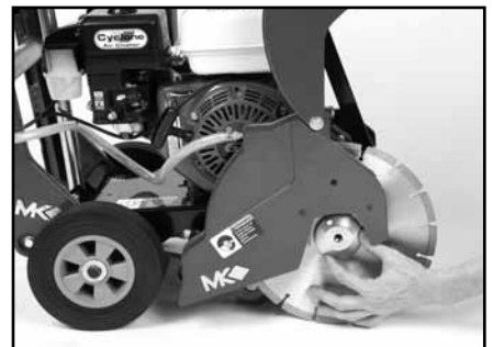
(F) Install the Outer Flange. Verify it is seated against the blade.
