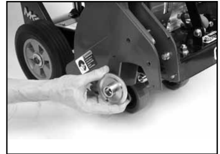
(I) Install the Inner Blade Flange, Blade, Outer Flange and Blade Retaining Bolt.
