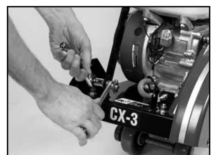
(L) Remove the Pointer.
