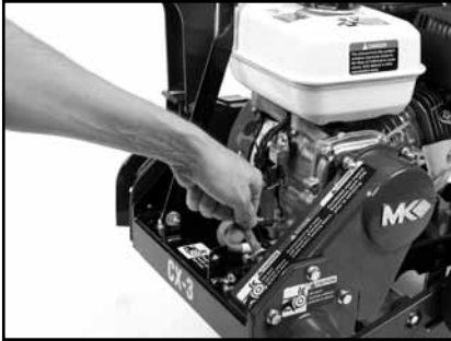
(P) Install the Belt Guard and Belt Guard Retaining Bolts.
