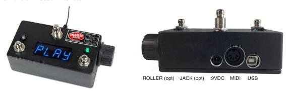
The DMC-3XL Gen2 and DMC-4 Gen2 are available with an optional side roller that sends expression or other MIDI data. If a pedal or switch is plugged into the expression jack, the roller will be disabled.
