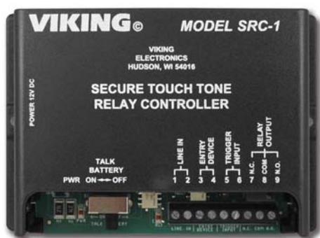
The **SRC-1** enables a standard touch tone phone to securely operate a set of timed relay contacts to control a doorstrike or gate controller at a remote location. The **SRC-1** is fully user programmable and uses non-volatile memory. The **SRC-1** eliminates the possibility of dialing the activation code through the entry phone using a hand held touch tone dialer.
