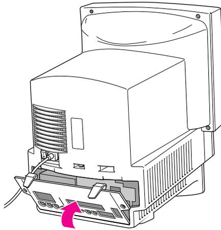
**16** If you removed security screws from the back panel in step 3, reinsert them.
