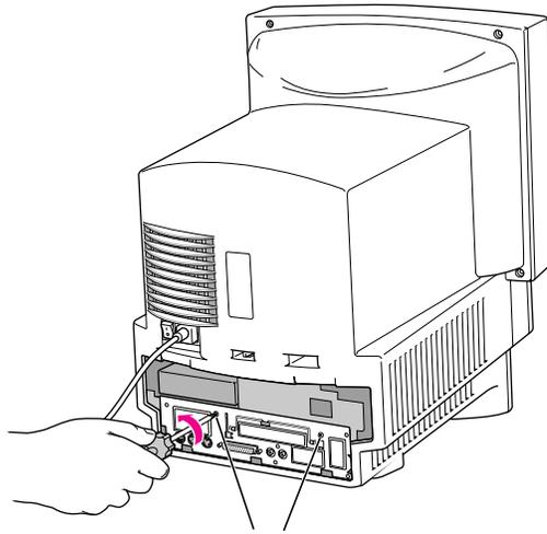
*Remove both retainer screws from the vertical plate.*
