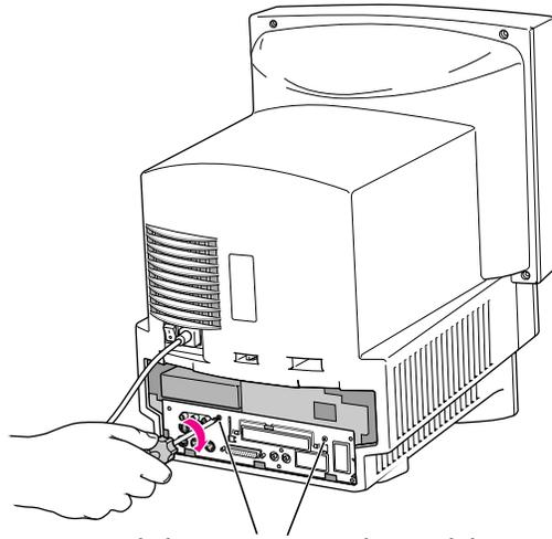
*Reinsert both retainer screws into the vertical plate.*
