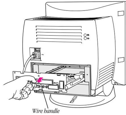
The logic board is plugged into a slot inside the computer. You may have to brace the computer with your other hand and pull firmly at first. Slide the entire logic board all the way out of the computer.
