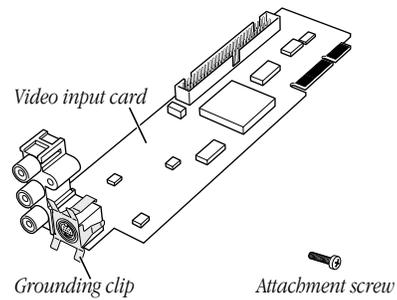
**Note:** The grounding clip may be a separate piece in your package. If so, you will attach it by following instructions later in the manual.
