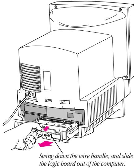
The logic board is plugged into a slot inside the computer. You may have to brace the computer with your other hand and pull firmly at first. Slide the entire logic board all the way out of the computer.
