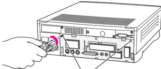
*If there are security screws, remove both screws from the vertical plate.*
