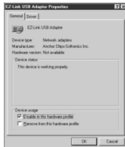
Figure 2.14 This sample network card Properties dialog box shows the status of the device.
