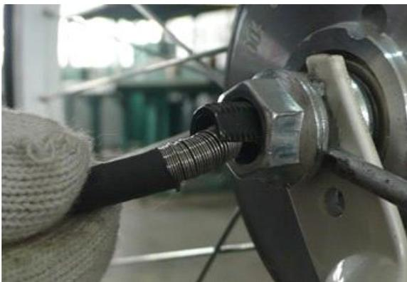
**IMPORTANT:** *Make sure that the torque washer fits firmly inside the fork dropt-outs and is completely stable. If the torque washer doesn't fit properly, contact a local bike service shop for assistance on finding a different washer or replacing the fork altogether. Remember that damage caused by motor "spin outs" is not covered by the warranty.*
