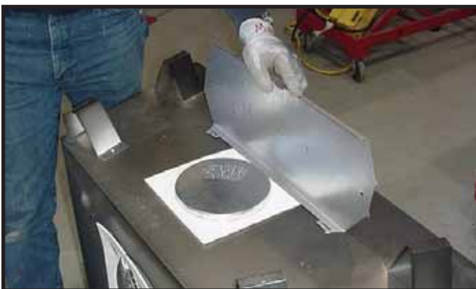
Figure 7.2 Rotate the top heat shield to the vertical position as shown above. The heat shield must remain in the vertical position.
