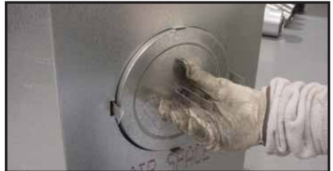
Figure 7.10 Fold the center parts of the retaining band out and use to remove the vent cap.
