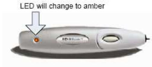
Position the reader in a perpendicular position to the tag and position the tip a few millimeters to one side of the tag, the optimal read range for most tags will be 0-2cm.
