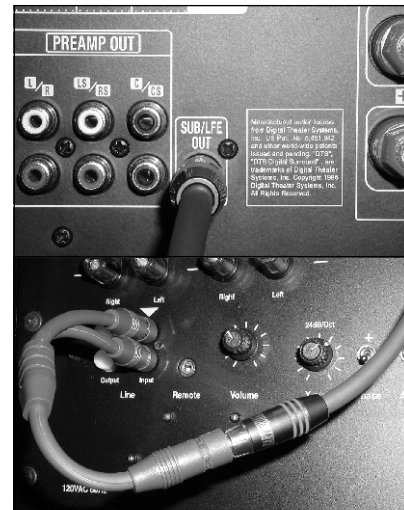
RCA connection from Processor to SuperNova using a "Y" connector.
