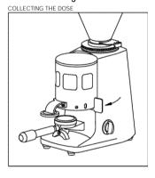
In order to release a portion of ground coffee, the doser lever must be pulled all the way and allowed to return on its own. Pull twice in a row for a double portion.
