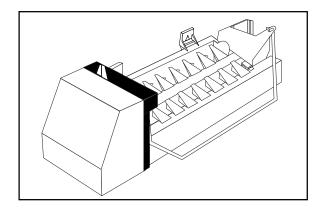
2. When frozen, the cubes are moved up and out of the mold. The sweeper arm ejects them into the ice storage bin below.
