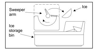
3. The feeler arm senses when the bin is full and signals the icemaker to stop ejecting more cubes. However, the mold has been refilled and cubes frozen so the new supply is ready when needed. As soon as ice is removed from the bin, the feeler arm signals that more is needed. Icemaker resumes operation by ejecting ready-and-waiting frozen cubes.
