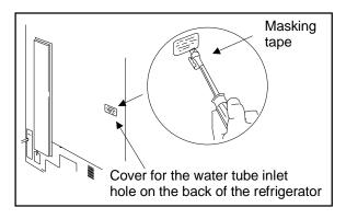
b. After removing the cover, use the screwdriver to pierce the interior sealing tape that covers the hole for the water fill tube inlet. Clear a path for the water fill tube.
