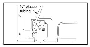
f. Plug the water valve wire connector into the terminal board at the points on the bottom right position, marked "1" and "2" across from "A" and "B".
