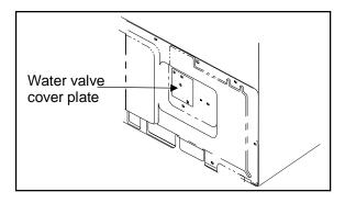
b. Remove wire harness attached to cover plate by squeezing wire tie with pliers and pushing tie through hole in plate. Pull end of wire harness through opening in back cover. Discard plate.
