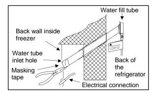
e. From the back, push gently on the water fill tube while twisting it slightly, until the flange is firmly seated on the hole on the back of the refrigerator. Make sure the water fill tube is completely seated.
