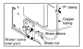
g. Secure the ¼" flexible copper tubing with the P-clamp at the back horizontal cover, using the existing cover screw. Create a service loop out of additional 8' of copper tubing.
