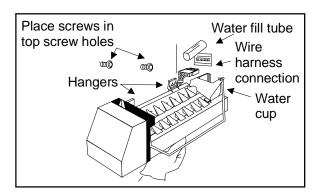
e. Slip the icemaker hanger over the mounting screws while easing the icemaker water cup toward the end of the water fill tube.
