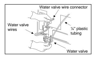
**e.** Attach the water valve to the lower rail using the hex screws removed from the mounting plate. This will assure that the water valve is electrically grounded.
