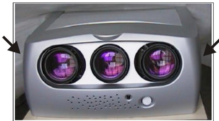
To remove the second top cover, covering the electronics, first the side covers have to be removed.
