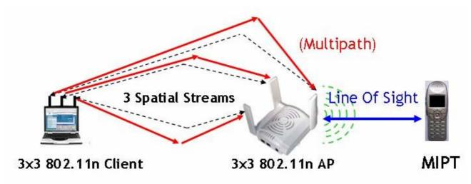
Figure 27: MIMO principle
