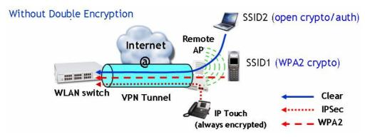
Figure 16: Encryption on Remote AP
