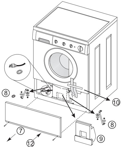
11. From the rear of the washer, carefully pull out the power supply cord through the hole in the backsheet.
