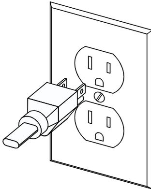
**OUTLET RECEPTACLE** - Properly grounded 3-prong receptacle to be located so the power supply cord is accessible when the washer is in an installed position. NOTE: GFI (Ground Fault Interrupter) receptacle is not required.
