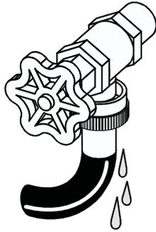
Carefully connect the other inlet hose to the inside "C" outlet of the water valve. Tighten by hand, then tighten another 2/3 turn with pliers.
