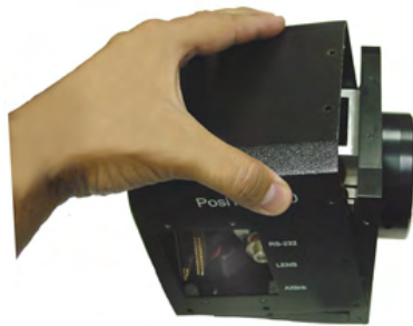
FIG. 8 Removing cover on the PT10 and PT15
