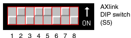
FIG. 5 AXlink device DIP switch (S5) (default value of 90)
