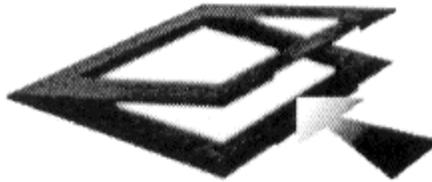
3. Lift up the Scanner's transparency adapter and place the Scan Frame on the scanner's object glass.
