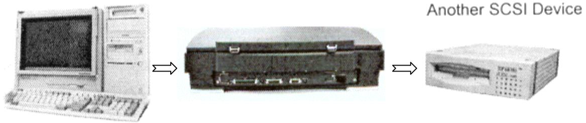
**Case 3:** Scanner is the *last* SCSI device in the SCSI Chain.
