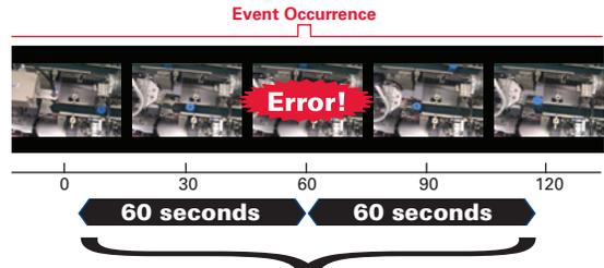
When a predefined event is triggered, video before and after the event (max. 120 sec.) is automatically recorded and stored as a log.
