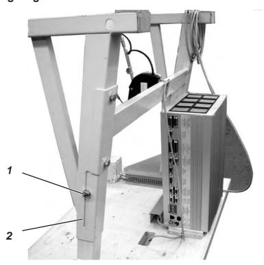
The working height is adjustable between 750 and 950 mm (measured up to the top edge of the table top).
