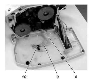
Fasten the oil lines 8 and 9 in the oil pan by means of fitting 10.
