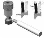
Unscrew the terminal. Thread the bared end of each cable through the hole in the bottom of the terminal post. Ensure that there are no loose strands which may touch adjacent terminals. Retighten the terminal securely.
