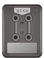
Quad crossover networks separate the treble and bass networks into two distinct sections, each connected by a dedicated pair of terminal posts. This enables the treble and bass components to be separately driven for optimum performance. The upper pair of terminals is connected to the treble network and the lower pair to the bass network.
