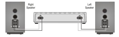
Choose a suitable length of twin core speaker cable for each channel, and prepare the ends as described above.
