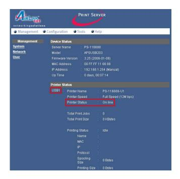
**Step 5** Click on the **Tools** link, select the port you want to test and click the **Test** button. The Print Server will perform a low-level print test, bypassing the operating system layer.
