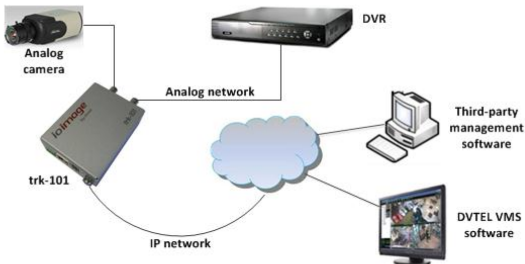
Figure 2: trk-101 Unit Connectivity
