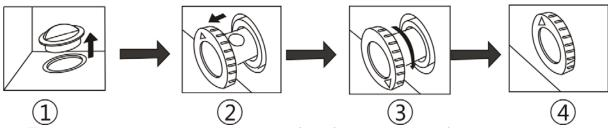
1. There is a water conduit at the bottom of the freezer, when defrosting, extract the
