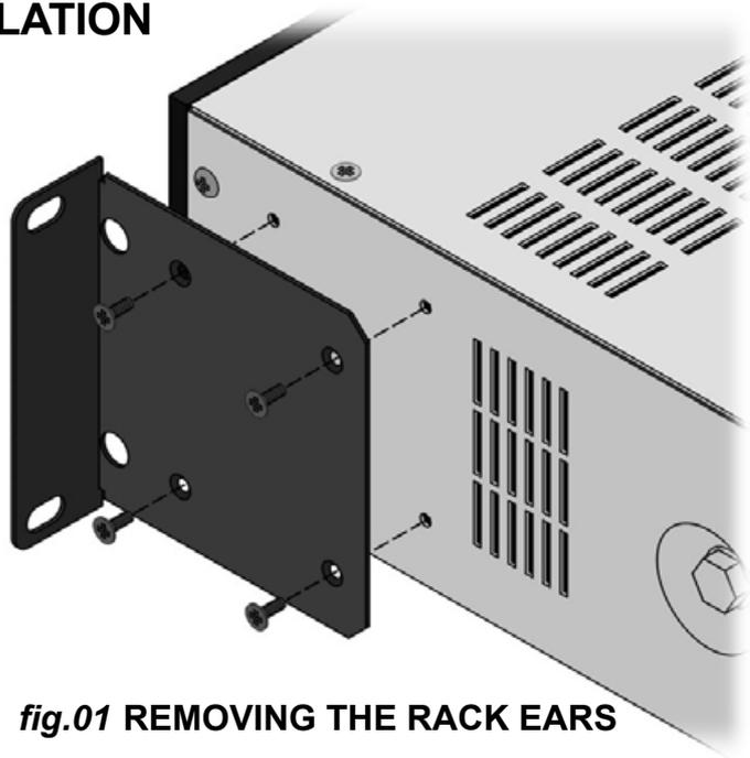
**fig.01 REMOVING THE RACK EARS**
