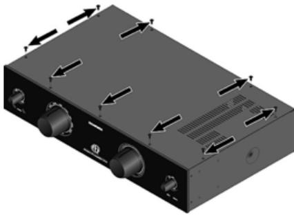
A few of the factory default settings can be altered via jumpers inside the unit to customize to your absolute optimum functional preferences. The following procedure must be done with great care and by a competent professional. Before continuing turn the power off and remove the mains I.E.C. cable. To gain access to the jumpers you must first remove the cover - this is done by unscrewing the nine screws, positioned as shown left:
