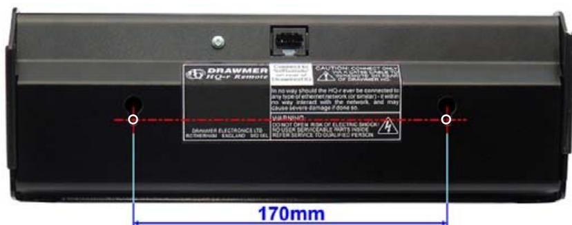
The remote can be fixed to a desk to provide further stability via the the two holes on the bottom of the unit. Screw in to a desk two screws at a distance of 170mm apart and to a depth of 5mm to the shoulder, then slot the remote over the holes.
