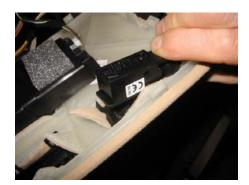
Above, right, is the mic as you are ready to press it into the grill. Note that the arrow on the back of the mic should point toward the front of the vehicle.
