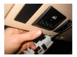
Next, locate the correct three conductor wire (below left). It will be a black connector and should have one wire that is clear in color. You may need to do some fishing for it on either side of the opening. Detach the wire from the cable holders so that you have enough wire to reach where the mic goes. Connect the microphone.
