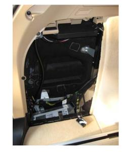
For convertible E46s you will find the connector behind the drivers side back seat seatback. Access will be via a small silver metal "hatch."
