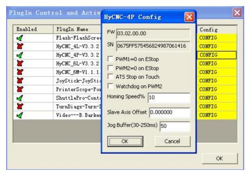
Tick "Watchdog on PWM2" to enable the watchdog function. When Mach3 works properly, PWM2 output a 50% duty cycle signal. When Mach3 works abnormally, PWM2 output a 0 duty cycle signal. When watchdog is enabled, PWM2 can't be controlled by a M code. As soon as watchdog is enabled, it can't be disabled until USB interface's power is recycled. To disable the watchdog, untick "Watchdog on PWM2", exit Mach3, recycle the USB interface's power and restart Mach3.
