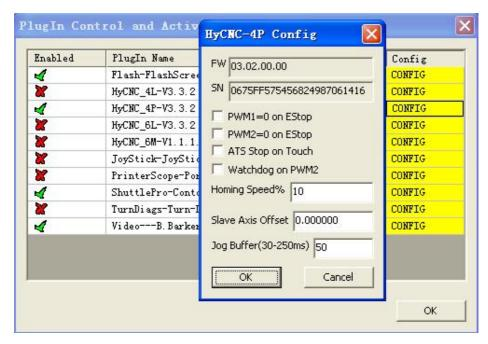
FW is the firmware version and SN is the hardware serial number.
