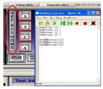
DoButton(22), DoButton(23), DoButton(24), DoButton(25), DoButton(26), DoButton(27) are used to execute auto zero on X/Y/Z/A/B/C axis. The above script execute homing on Z axis, then Y axis, then X axis and finally A axis.
