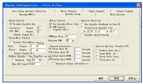
Then click Apply and OK to close the config window. Then switch to page "Diagnostics" of the Mach3's main interface and type "M7 $\checkmark$ " to switch on mist,
