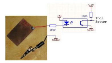
There is an improved low cost tool setter shown in the figure below. It requires the same connection and optical coupler circuit as the low cost tool setter described above. However, its setting method should be as same as the professional one.
