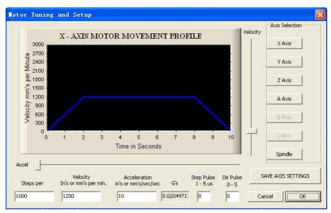
Click on "X Axis" button on the upper right corner. Then fill in "Ster per" (mm/inch) according to the following equation
