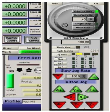
The jog response speed can be adjusted by "Jog Buffer" length in "HyCNC-4P" plugin's "CONFIG" setting. The smaller the buffer is set, the faster response speed becomes. However, the larger chance of inconstant motion caused by PC OS's scheduling timing error.
