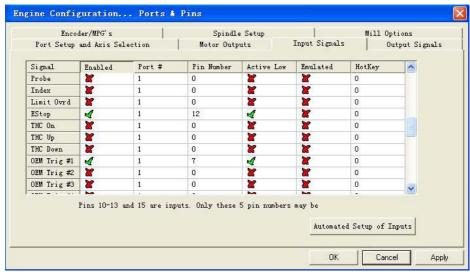
When EStop is trigged, the GCode execution is stopped. If 2 PWM outputs also required to stop, put "X" on "PWM1=0 on EStop" and "PWM2=0 on EStop" in "HyCNC-4P Config" window. The "HyCNC-4P Config" window can be shown by operating the main menu "Config"->"Config PlugIns".
