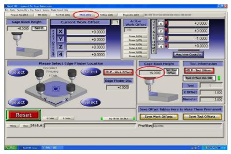
Finally, script for auto tool setting needs to be updated. Operate the main menu "Operator"->"Edit Button Script". Then click on flashing "Auto Tool Zero" button, as shown below.
