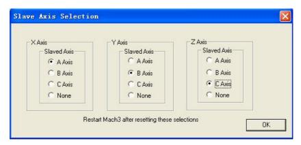
When homing is carried out with a slave axis, machine seeks both home switches on the main and slave axis in the first stage. When both switches are triggered, machine decelerates to 0 and the second stage start. The machine also checks both homing switches in the second stage. The alignment error between the main and the slave axis is compensated during the deceleration stage. The alignment offset can be adjusted "Slave Axis Offset" in "HyCNC-4P" plugin's "CONFIG" setting.
