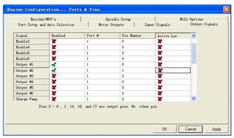
Coolant control can be used to test "Output #1" and "Output #2". Click on page "Spindle Setup". Set as the following figure for "Relay Control" and "Coolant Mist Control" blocks, in which "Output #1" is used to control mist and "Output #2" is used to control coolant.
