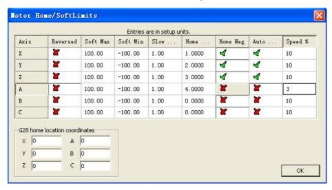
The first stage speed is defined by "Home Speed%" in plugin's config. Operate Mach3 main menu "Config" -> "Config PlugIns".
