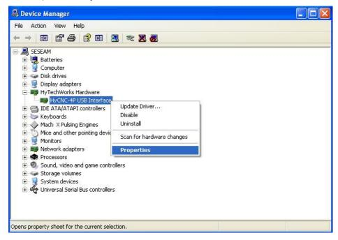
Then click "Details" page and select "Device Instance Id". The last 8 characters following the VID and PID number is the USB serial number.
