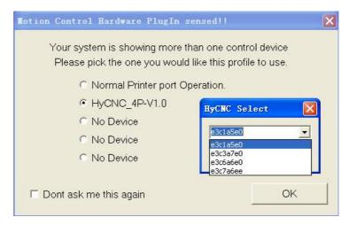
The firmware version and the hardware serial number of the HyCNC-P cab be read by operate Mach3 main menu "Config"->"Config PlugIns".
