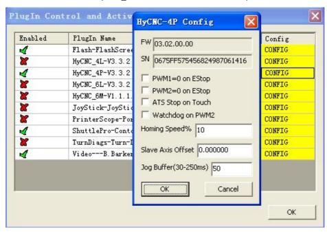
Putting "X" before "ATS Stop on Touch" selects auto tool setting using low cost tool setter. Removing "X" before "ATS Stop on Touch" selects auto tool setting using professional tool setter.
