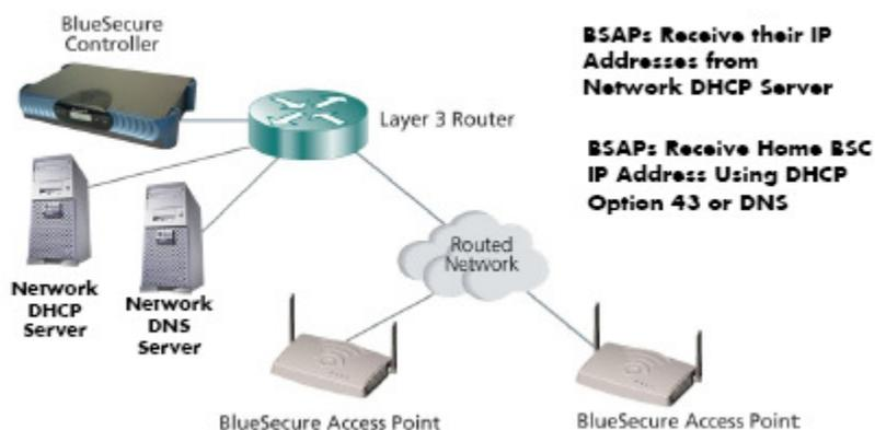
**Figure 3: Deploying BSAPs across a routed network**
