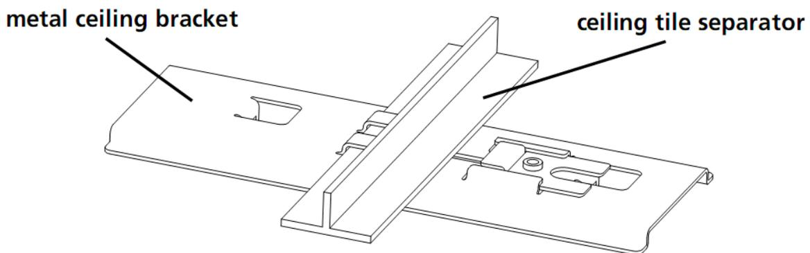
3. Slide the moveable section into place and tighten the screw (found underneath) to secure it.
