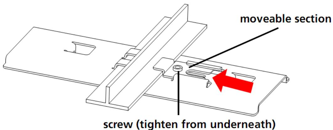
4. Position the BSAP-1800 so that the two tabs from the ceiling bracket locate in the slots in the BSAP-1800 (A), then slide the slider across to lock the BSAP-1800 to the bracket (B).
