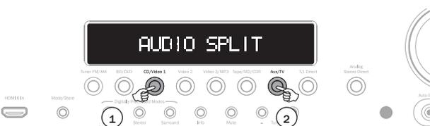
The 551R V2 allows splitting from any source whatever its video input type but only to sources where analogue or digital audio is the current audio input type, not HDMI.
