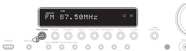
1. Press the *Tuner FM/AM* button on the front panel or remote control to select Tuner mode.
