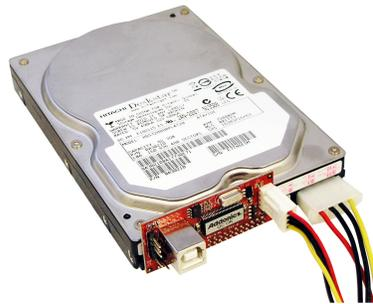
5. Now connect the B-type USB cable to the USB port on the converter or use the USB pin header cable.
