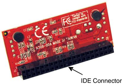
Note: It is required to set up the IDE hard drive you are connecting to the converter as a MASTER device.
