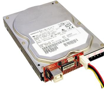
4. At the other end of the Y-power cable is the 4-pin Molex power connector that you connect to the hard drive.
