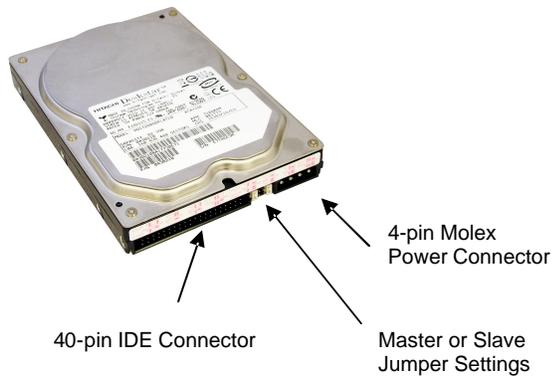
2. Connect the converter board to the IDE connector of the hard drive.
