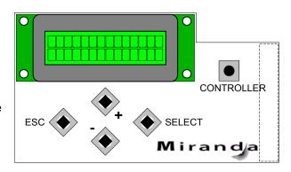
The local control panel displays a menu that can be navigated using the four pushbuttons located beneath the display. The functionality of the pushbuttons is as follows:
