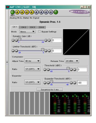
The *Dynamic Gain* is adjusted from 0 to +24 dB gain with the slider or a direct keyboard entry.
