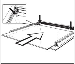
Push the middle pane into the frame almost to the end. Fit the sealing strip into position, then push the pane in as far as it will go.
