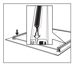
■ Fit the side seals for the inner pane in the grooves provided.
