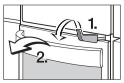
The lock is fitted beneath the control panel to prevent the door from being opened. The door can only then be opened by pressing the lever.
