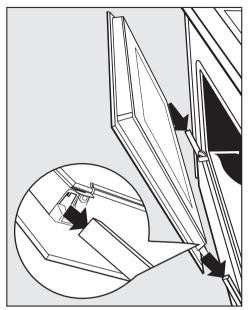
Hold the door securely at both sides and carefully fit it back onto the hinge guides.
