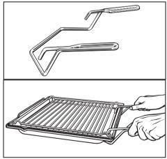
The handle makes it easier to take the tray and rack out of the oven, or to put them into it. The two prongs at the top go inside the tray or over the top of the rack and the U-shaped supports underneath.
