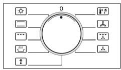
The function selector is used for selecting your cooking function. It can be turned clockwise or anticlockwise.
