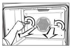
Remove the screws in the back panel and take it out.
