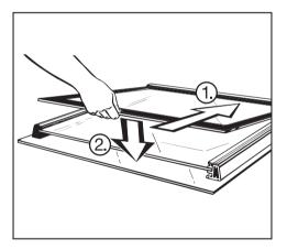
Insert the inner pane with the printed text facing downwards.
