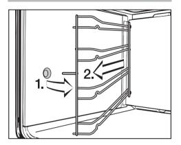
Pull the runners to the side and then forwards. Remove the catalytic side panels (if present) at the same time.
