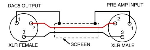
**CONVENTIONAL: SCREEN CONNECTED AT BOTH ENDS**
