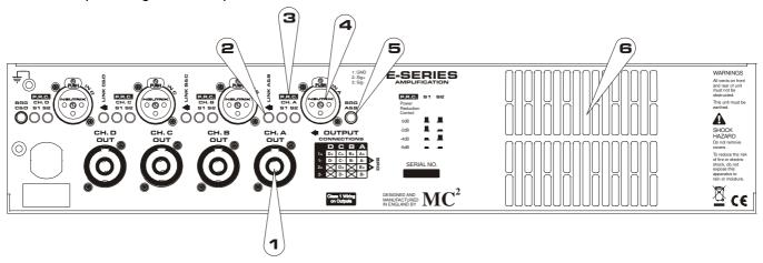
1: Channel A output Speakon socket: Normal output is on pins 1+ hot, 1- cold. Channel B's output is also wired to this socket to enable a single NL4 to provide both channels and to facilitate easier wiring in bridged mode. Channel B is wired pins 2+ hot, 2- cold.
