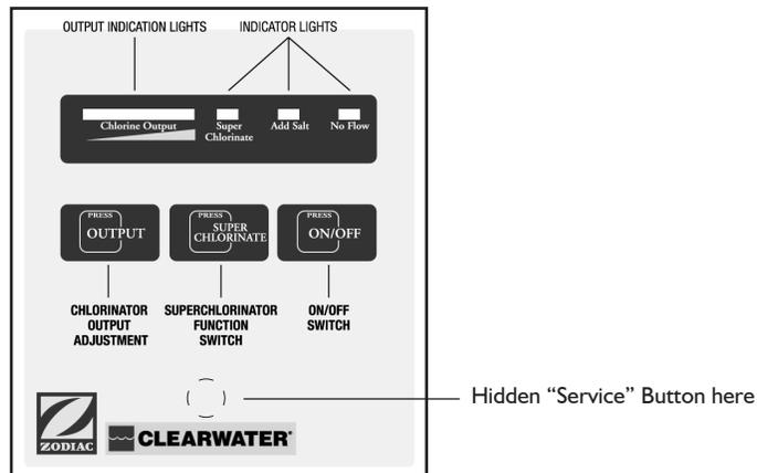
4. Continue to hold the "service" button down until the correct number of flashes for the controller being used is observed. See the controller chart below.
