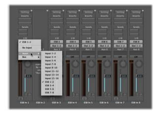
Logic Pro 8 handles mono and stereo channel settings separately. This means that you can set up the ESB inputs for eight mono channels, and then switch the audio channels to stereo operation. Once the desired DTDM output channels are set appropriately for each aux input, save your project as a template. This will allow you to switch quickly between mono and stereo setups, without needing to manually change settings each time.
