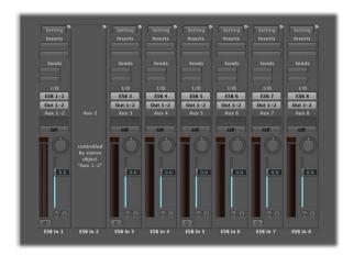
Within mono aux channel strips, you can select the desired output channel of the DTDM Mixer (ESB 1–8). Stereo aux channels can be set to input channel pairs ESB1–2, 3–4, 5–6, and 7–8. Please take a closer look at the available inputs:
