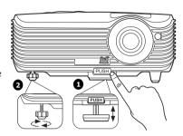
If the projector is not placed on a flat surface or the screen and the projector are not perpendicular to each other, the projected image becomes trapezoidal. To correct this situation, see "Correcting keystone" on page 25 for details.
