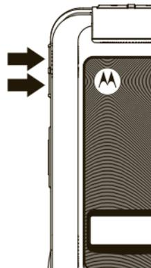
**Tip:** You can quickly set your ringer to **Vibrate All** by holding the down volume key in the home screen.
