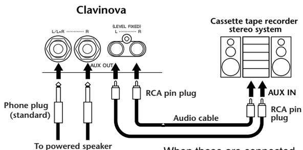
When these are connected (with standard phone plugs), you can use the [MASTER VOLUME] control to adjust the volume of the sound output to the external device.
