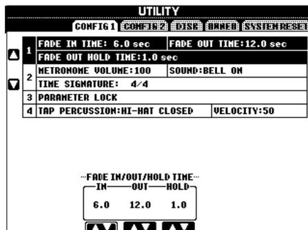
Determines the time it takes for the volume to fade in, or go from minimum to maximum (range of 0 - 20.0 seconds).
