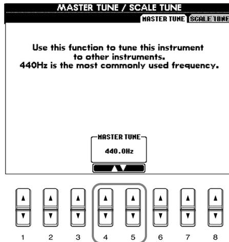
Determines the overall pitch of the CVP-205/203, from 414.8 - 466.8 Hz. Press the 4 or 5 [▲▼] buttons simultaneously to instantly reset the value to the factory setting of 440.0 Hz.
