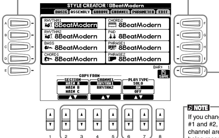
**2** Selects the style section and channel that will be copied to the corresponding channels, selected with the [A]-[D] and [F]-[I] buttons above.
