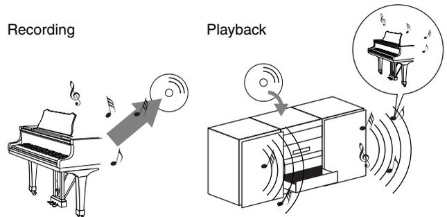
In the above example, the actual acoustic sounds of the pianist's performance are captured in the recording as audio data, and this is recorded to CD. When you playback that CD on your audio system, you can hear the actual piano performance. The piano itself is not necessary, since the recording contains the actual sounds of the piano, and your speakers reproduce them.
