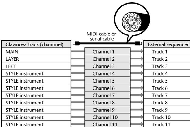
As you can see, it is essential to determine which data is to be sent over which MIDI channel when transmitting MIDI data (page 138). The Clavinova also allows you to determine how the received data is played back. (page 139).
