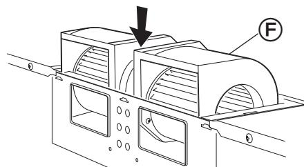
Reattach blower unit to back of microwave hood cabinet with two screws removed in Step 3.
