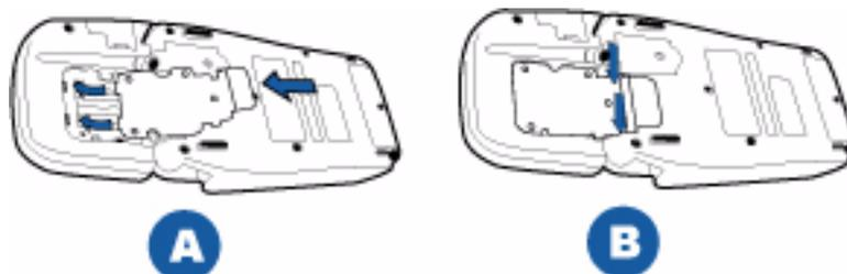
**Figure 9** Installing the Metal Plate
