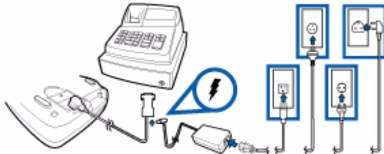
Figure 17 RS-232 Connection with External Power Brick
