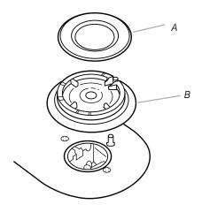
A. Burner cap B. Burner
