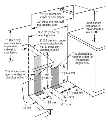
**NOTE:** 24" (61 cm) minimum when bottom of wood or metal cabinet is protected by not less than  $\frac{1}{4}$ " (0.64 cm) flame retardant millboard covered with not less than No. 28 MSG sheet steel, 0.015" (0.4 mm) stainless steel, 0.024" (0.6 mm) aluminum or 0.020" (0.5 mm) copper.
