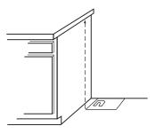
If the cabinet opening is wider than specified in the "Location Requirements" section, adjust the template so the range will be centered in the cabinet opening.
