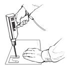
To mount the anti-tip bracket to a concrete or ceramic floor, use a 3/16" (4.8 mm) masonry drill bit to drill 2 holes at the positions marked on the bracket template. Remove the template from the floor.
