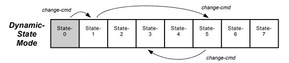
**Caution:** in Dynamic-State mode, any changes to the *Current-State* are immediately saved, so you do not want to allow a user to change to a state that is storing a preset or paging configuration – you are relying on preset and page states to be static after they are programmed.
