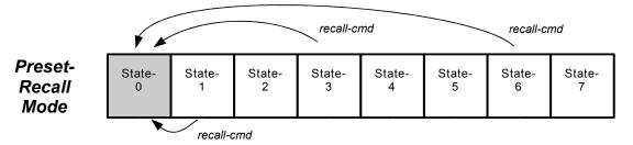
Each of these *Presets* store a completely different configuration of the machine, and since they are recalled (copied) into state-0, the presets are not changed if you subsequently change routes, volumes, etc. However, previous routes on all zones in state-0 are lost (unlike a page, where the previous state is restored).
