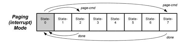
This diagram shows paging from State-0, but note that if you are currently in another state (Dynamic-mode), the paging function works the same, restoring the original state.
