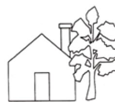
Trim or remove any nearby trees that would interfere with the chimney draft.
