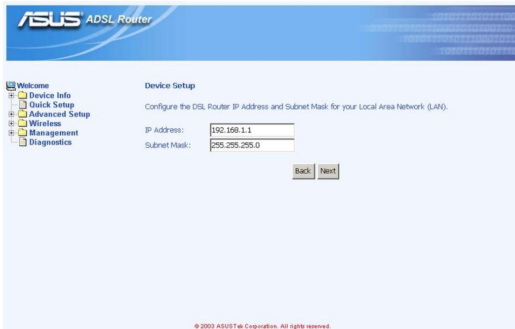
**Figure 5.3 Setup IP address and subnet mask**
