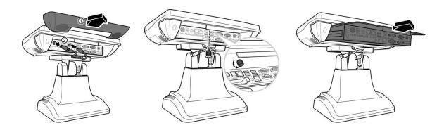
3.6 Replacing Hard Disk Drive
