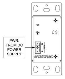
Hardware Connections for the TPMC-3X-DSW (Side View)
